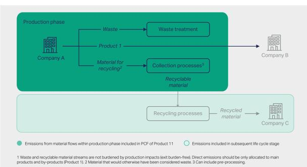
Figure 11: Allocation of waste treatment and recycling emissions
