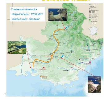
13 dams 21 power plants 2000 MW (peak) 6500 GWh/yr 250 km channel Watershed:11 700 km2 Average flow: 180 m3/s (min. 30 m3/s) Flash flood: 2700 to 6000 m3/s (1994/1882)
